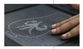
Dot Pad is compatible with many Apple devices (iOS & iPadOS 15.2 and higher) and integrates with VoiceOver to provide additional screen reading capabilities. Connect to iPhone or iPad via Bluetooth or USB-C cable (no additional apps required).
