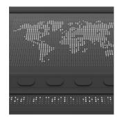
It instantly converts any input on a connected device into a tactile graphic – including handwriting, sketches, signatures, graphs, maps, diagrams and photos – that you can interact with and explore in detail.
